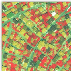
NIR2 – Yellow – Blue Roof Material Identification
